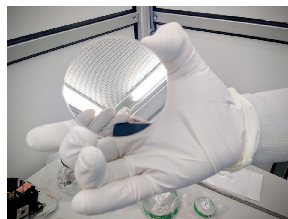
The new dichroic entrance which will let infrared light enter the cold part of the instrument and reflect optical light to the adaptive optics system.
